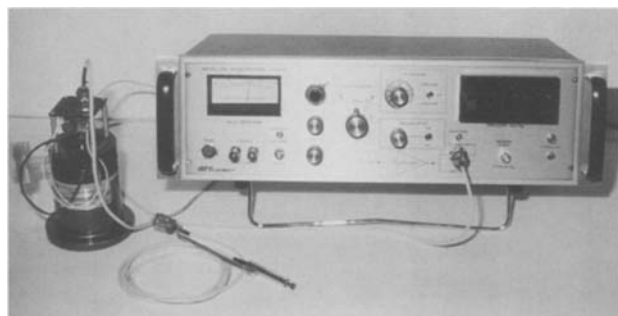
Fig. 3. The model 900 micropressure system includes microelectrode holders, preamplifier with active probe, power amplifier, hydraulic servo system, pressure transducer, and digital pressure readout
